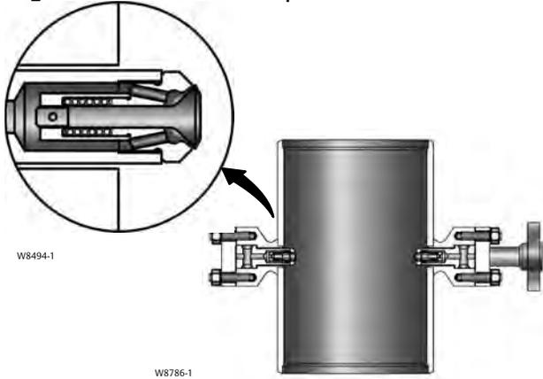
Figure 4. Detail of Spray Nozzle
