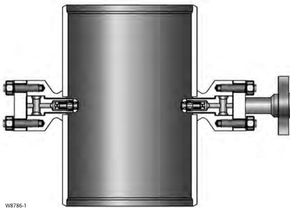
Figure 2. Fisher TBX-T Desuperheater with Optional Liner
