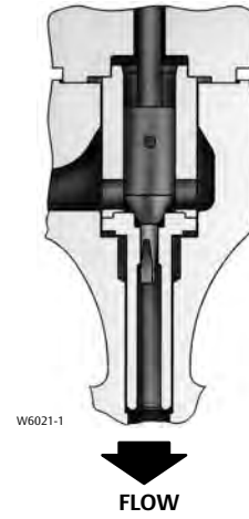
Figure 14. Fisher HPAS Trim with Micro-Flat Valve Plug
