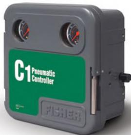
**Pneumatic Controllers** are mechanical devices designed to measure temperature or pressure and transmit a corrective air signal to the final control element. Bourdon tubes, bellows, temperature elements, or displacers are used as the sensing elements. The power supply and output of a pneumatic controller is compressed air or natural gas. ▶ 4194 | 4195K | 4196 | 4660 | C1
