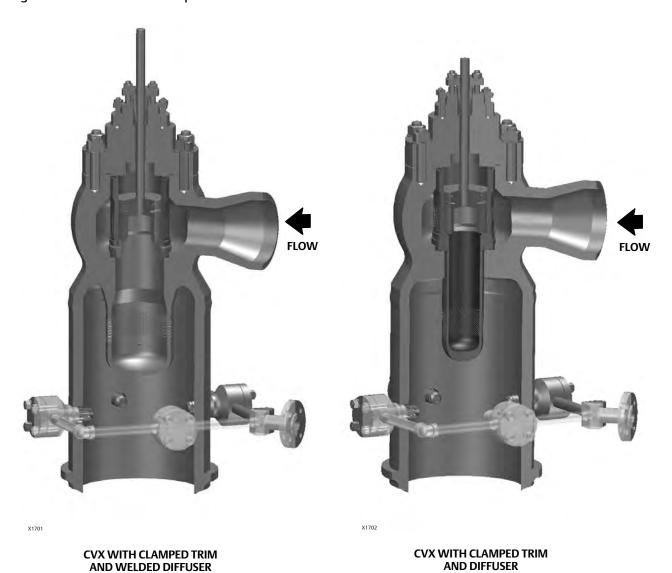
Figure 3. Fisher CVX Bore Seal Trim in Closed Position
