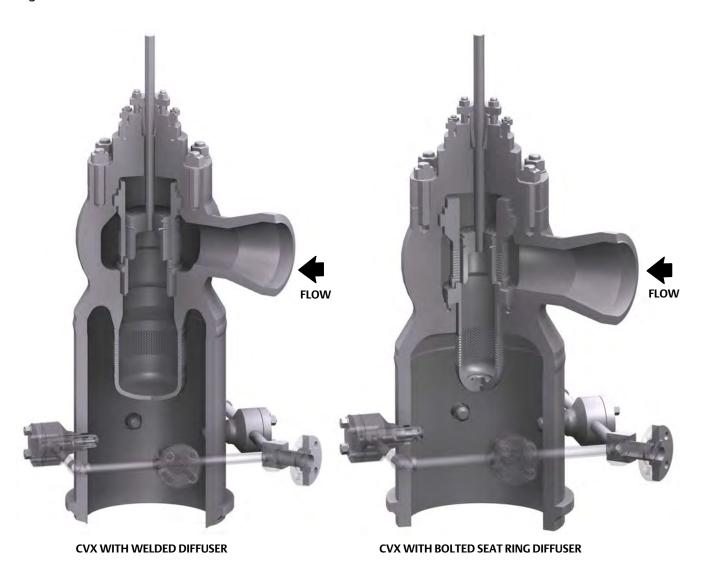
Figure 2. Fisher CVX with Clamped Trim
