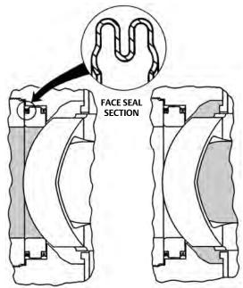
FORWARD FLOW SHUTOFF REVERSE FLOW SHUTOFF 4283375-A
