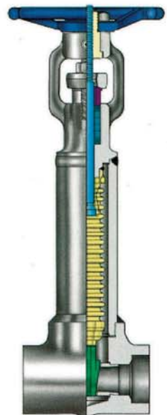
Bellows seal gate Class 800 ~ 1500 Flange ASME Class 150 ~ 1500
