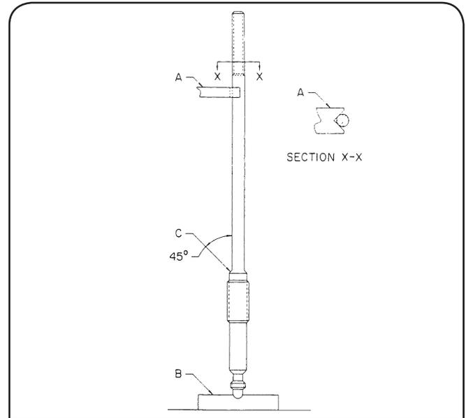
Figure 19: Spindle Runout Determination
