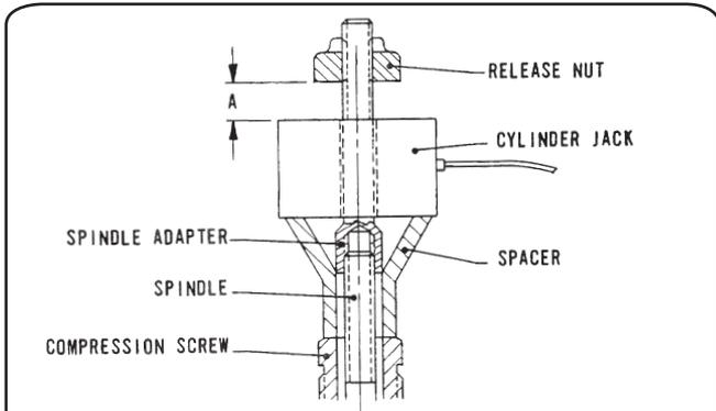
Figure 12: Hydraulic Assembly Tool
