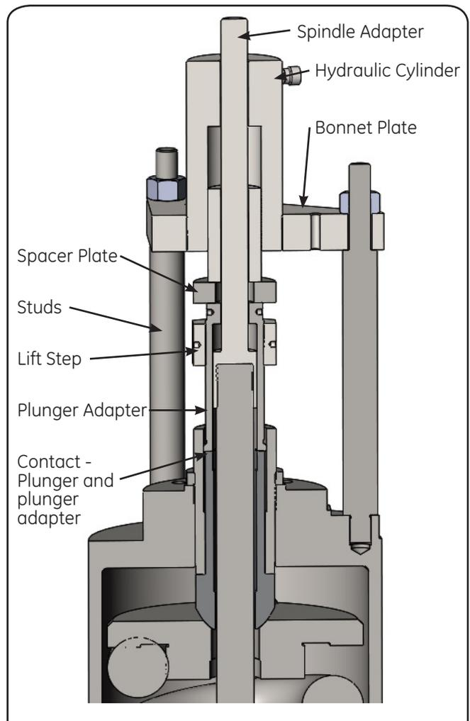
**Figure 34B: Hydraulic Set Device Settings for Set Pressure Adjustment**
