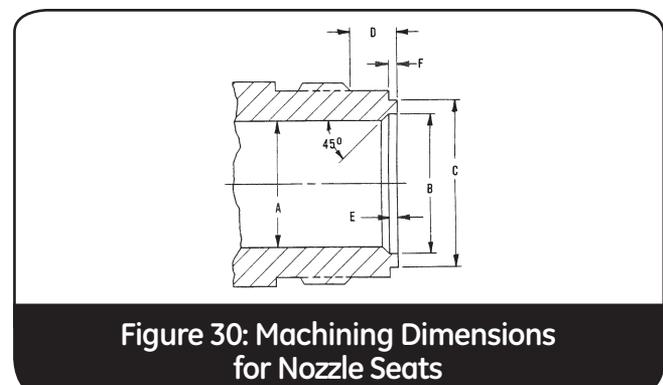
Figure 30: Machining Dimensions for Nozzle Seats
