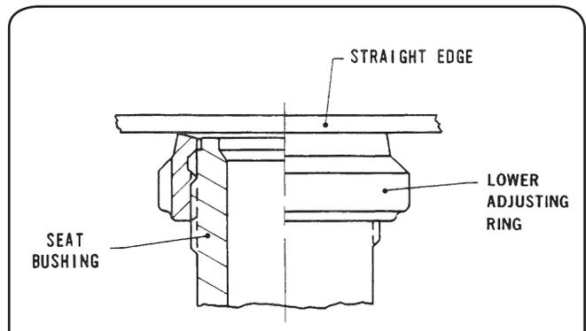
Figure 16: Checking Position of Lower Adjusting Ring
