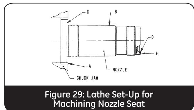
Figure 29: Lathe Set-Up for Machining Nozzle Seat
