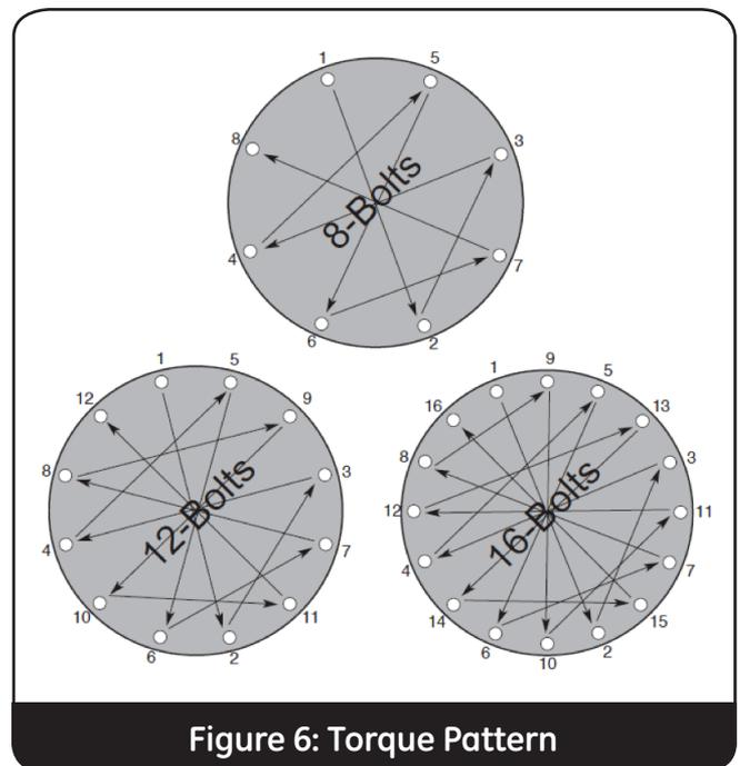
Figure 6: Torque Pattern
