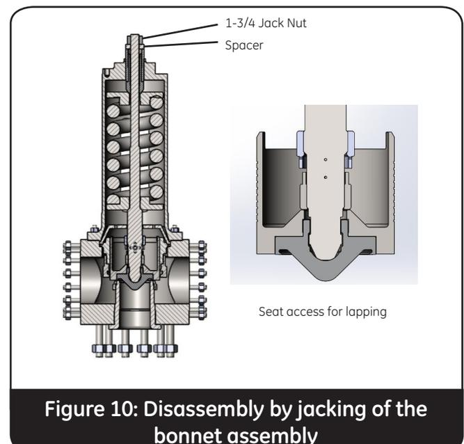
**Figure 10: Disassembly by jacking of the bonnet assembly**
