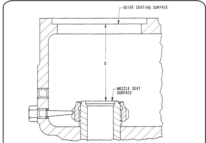
Figure 15: Nozzle Height Measurement
