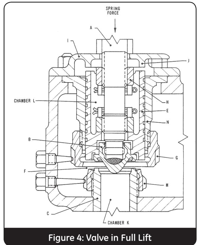
Figure 4: Valve in Full Lift
