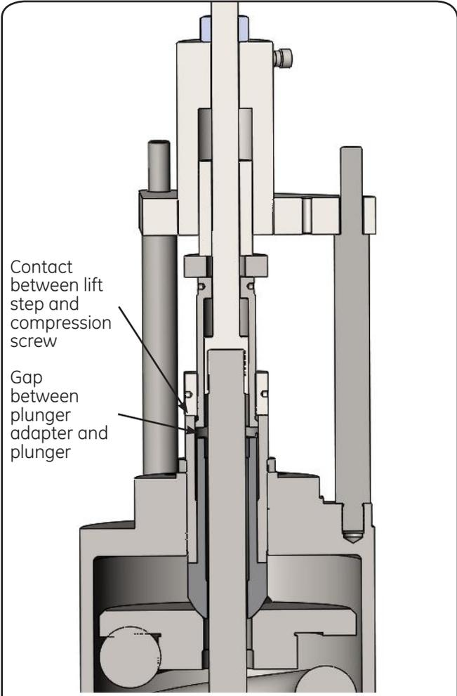
**Figure 35B: Hydraulic Set Device Settings used as an Auxiliary Lift Device**
