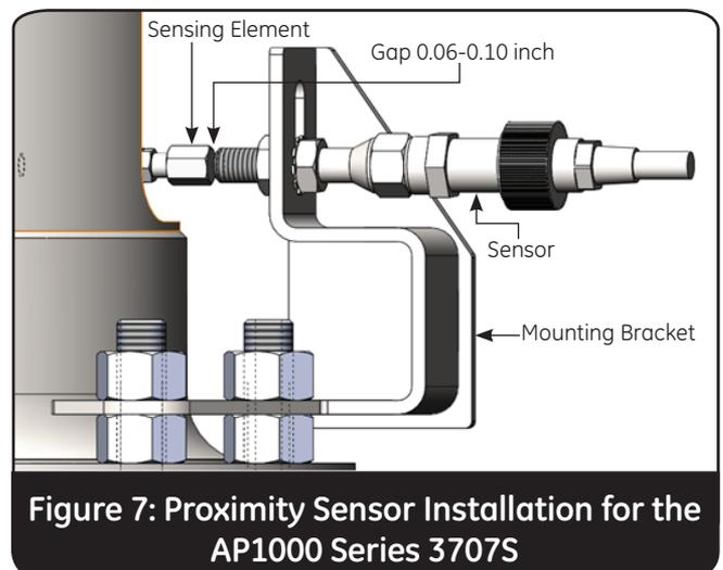
Figure 7: Proximity Sensor Installation for the AP1000 Series 3707S
