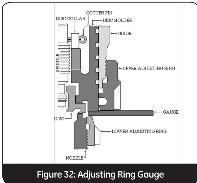
Figure 32: Adjusting Ring Gauge
