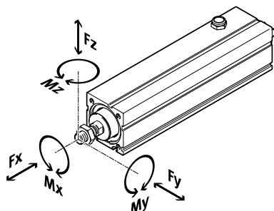
If there are two or more forces and torques simultaneously acting on the piston rod, the following equations must be satisfied:
