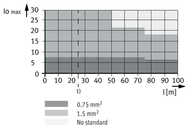
1) Cable lengths > 25 m possible following technical clarification; up to 99.9 m on request.
