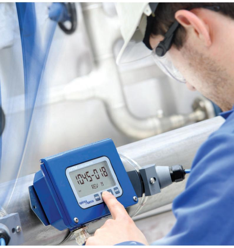
Please note: The UTM10 should not be strapped directly onto the pipeline if it is above 85°C.
