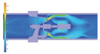
The compact wafer design of the Gilflo ILVA flowmeter also means that its installed length is much shorter than almost any other technology. It can be installed close to pipe bends, valves or other components that would prevent other types of flowmeter being fitted, as shown in the diagram below.
