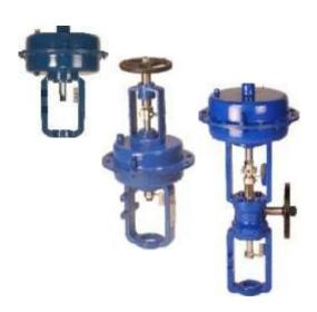
The 'M' Series control valve actuators are diaphragm actuators with pre-compressed multispring construction. They are compact, comparatively with less number of parts, easy to maintain, quickly reversible. The actuators are suitable for regulating and on-off applications. Various models are available covering small to larger thrust requirements.
