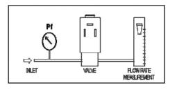
REFERENCE CURVE WITH AIR - Inlet pressure **P1 = 6.5 bar** REFERENCE COIL 24V DC - (SEE NOTE "A")
