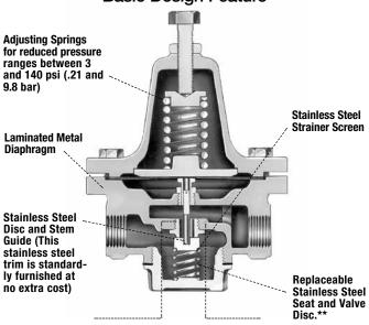
\*\* When utilizing a Teflon valve disc in the 152AT, the maximum operating temperatures are 300°F at 300psi (149°C at 21 bar) and 400°F at 200psi (204°C at 14 bar).
