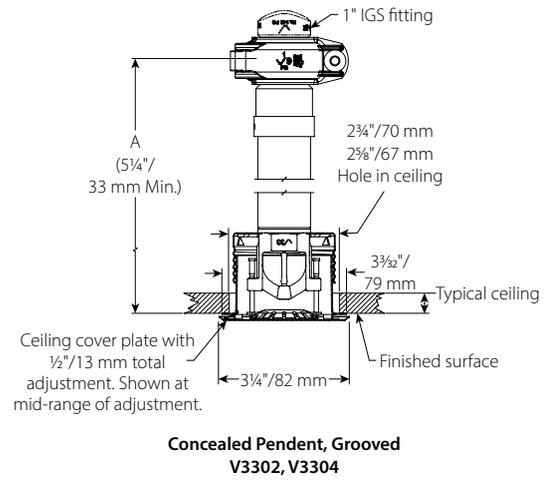
For wet system installation or dry/preaction systems installed in areas above 40°F/5°C
