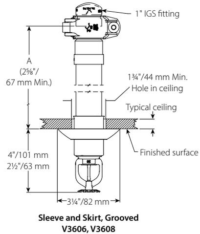
For wet system installation or dry/preaction systems installed in areas above 40°F/5°C
