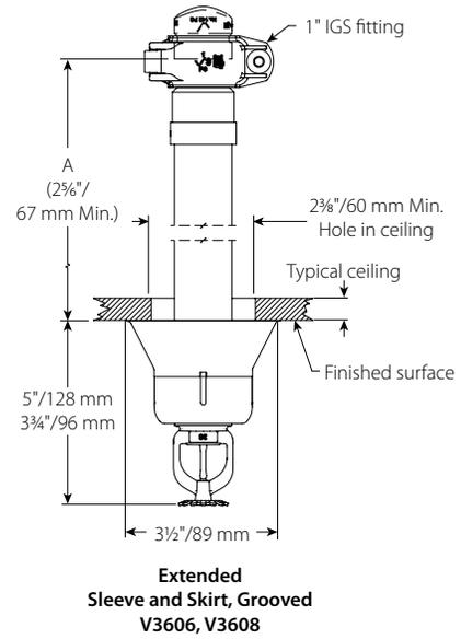
For wet system installation or dry/preaction systems installed in areas above 40°F/5°C
