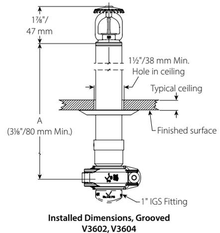
For wet system installation or dry/preaction systems installed in areas above 40°F/5°C
