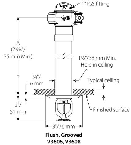
For wet system installation or dry/preaction systems installed in areas above 40°F/5°C
