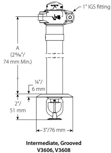
For wet system installation or dry/preaction systems installed in areas above 40°F/5°C
