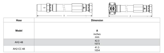
Note: Please reference section 5.0 Performance for complete list of Style AB6 Bracket listing and approval information with Series AH2-CC and Series AH2 lengths.
