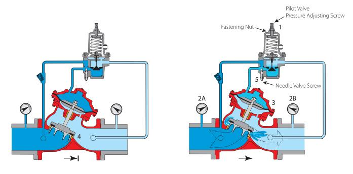
Valve Closed (static condition)
