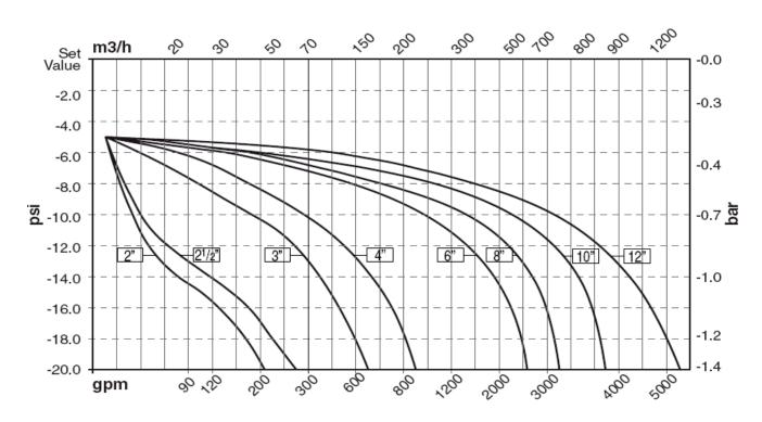
Table 2: Valve Outlet Pressure Fall-Off Characteristics Below On Inlet Under Set Pressure
