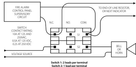
NOTE: The above diagram shows a connection between the common terminal (yellow – S1 and yellow-with-orange stripe – S2) and the normally closed terminal (blue – S1 and blue-with-orange stripe – S2). In this example, the indicator light and alarm will stay on until the valve is fully open. When the valve is fully open, the indicator light and alarm will go out. Cap off any unused wires (e.g. brown with orange stripe).
