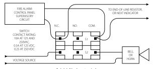
Switch 1: 2 leads per terminal Switch 2: 1 lead per terminal
