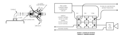
NOTE: The above diagram shows a connection between the common terminal (yellow – S1 and yellow-with-orange stripe – S2) and the normally closed terminal (blue – S1 and blue-with-orange stripe – S2). In this example, the indicator light and alarm will stay on until the valve is fully **CLOSED**. When the valve is fully **CLOSED**, the indicator light and alarm will go out. Cap off any unused wires (e.g. brown with orange stripe).
