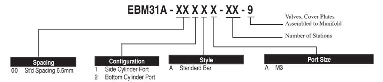
Note: Through ports (Inlet and Exhaust) are M7 Ports.
