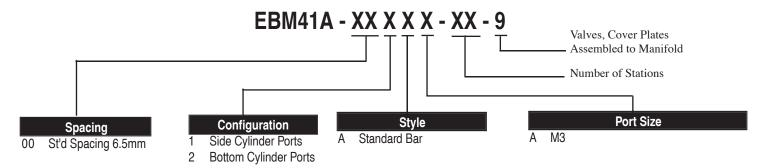
Note: Through ports (Inlet and Exhaust) are M7 Ports.
