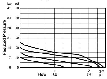
Reduced pressure range: 0 – 60psi (0 – 4.1 bar) Initial pressure: 100psi (6.9 bar)
