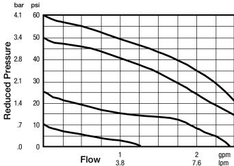
Reduced pressure range: 0 – 125psi (0 – 8.6 bar) Initial pressure: 100 – 150psi (6.9 – 10.3 bar)
