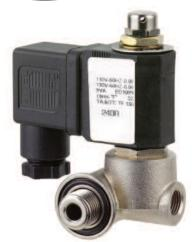
The Series PV three-way normally closed electro-pneumatic solenoid pilot valve effectively regulates supply pressures for the Series SAV Angle Seat Valve. The DIN connector is reversible 180 degrees to keep electrical wiring hassle-free, while the direct mounting banjo connection simplifies valve installation. Select the proper model according to the SAV valve actuator diameter and power requirements.
