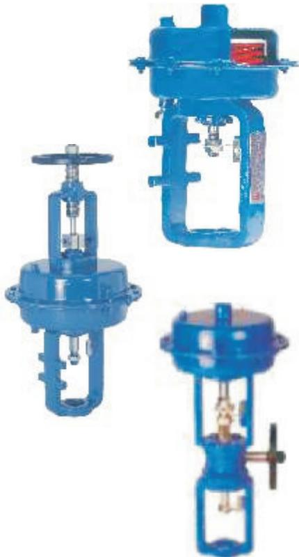
The 'M' Series control valve actuators are diaphragm actuators with pre-compressed multispring construction. They are compact, comparatively with less number of parts, easy to maintain, quickly reversible. The actuators are suitable for regulating and on-off applications. Various models are available covering small to larger thrust requirements.
