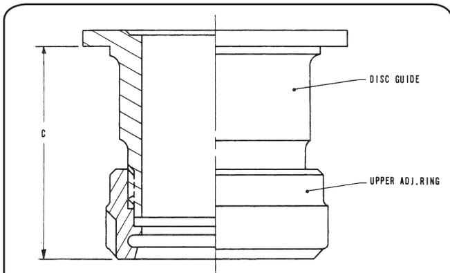
Figure 14: Checking Position of Upper Adjusting Ring
