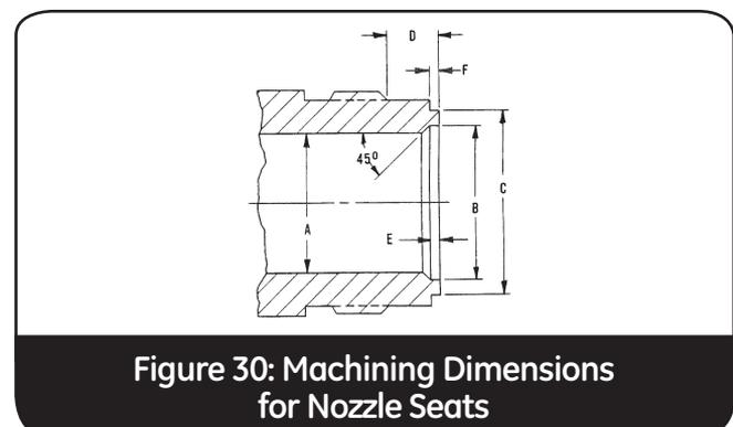
Figure 30: Machining Dimensions for Nozzle Seats
