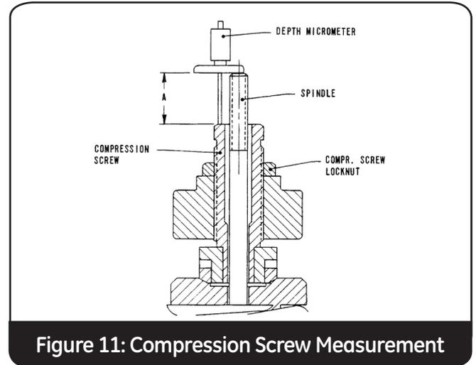
**Figure 11: Compression Screw Measurement**
