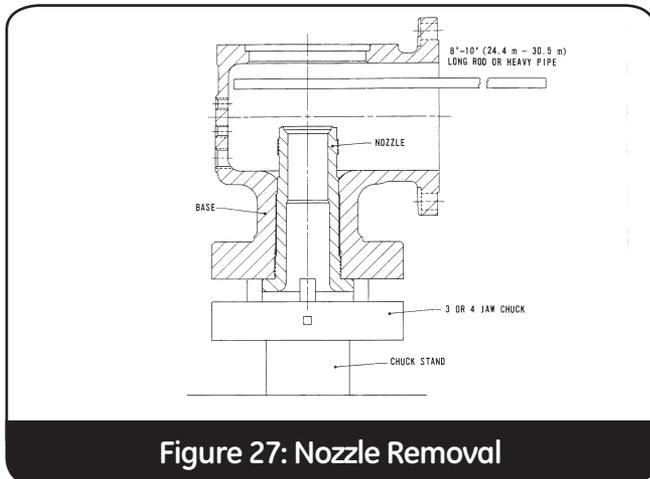
Figure 27: Nozzle Removal
