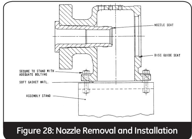
Figure 28: Nozzle Removal and Installation
