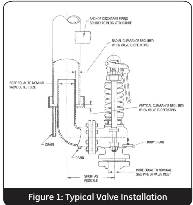
**Figure 1: Typical Valve Installation**
