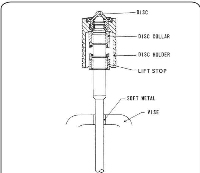
Figure 13: Disc-Spindle Assembly
