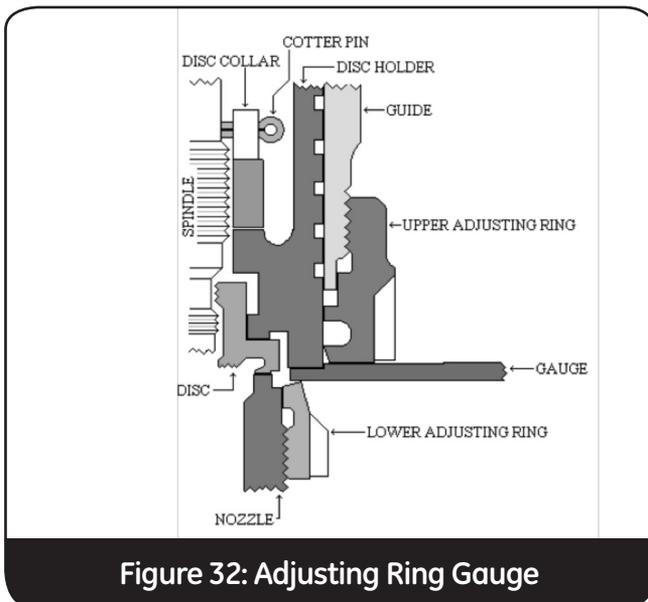
Figure 32: Adjusting Ring Gauge
