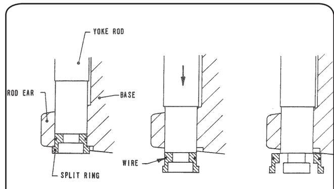
Figure 17: Removal of Yoke Rod
