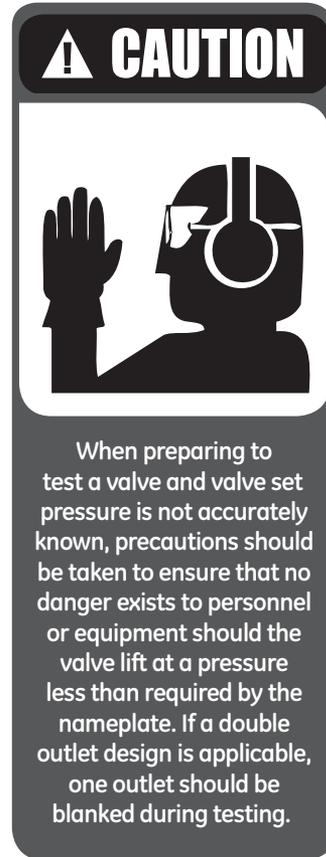
Bench testing ensures that the valve is capable of being set pressure adjusted and is leak tight.
