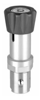
To meet the demands for the safe reduction of inlet pressures up to 6,000 psig, GO Regulator has designed the PR-56 Series regulator. This precision regulator features a piston sensing design which provides the operator with low adjusting torque requirements when setting the outlet pressure.
