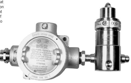
the HPR-2 vaporizing regulator. The heat exchange element uses GO Regulator's unique spiral wrapped screen as the heat exchange surface. This screen has up to 100 square inches of heat transfer area and precise design forces all sample flow to pass through the element just prior to exiting the regulator.
