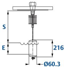
**Type 11D (one 4- or 8-contact switch mechanism and narrow switching differential)**
