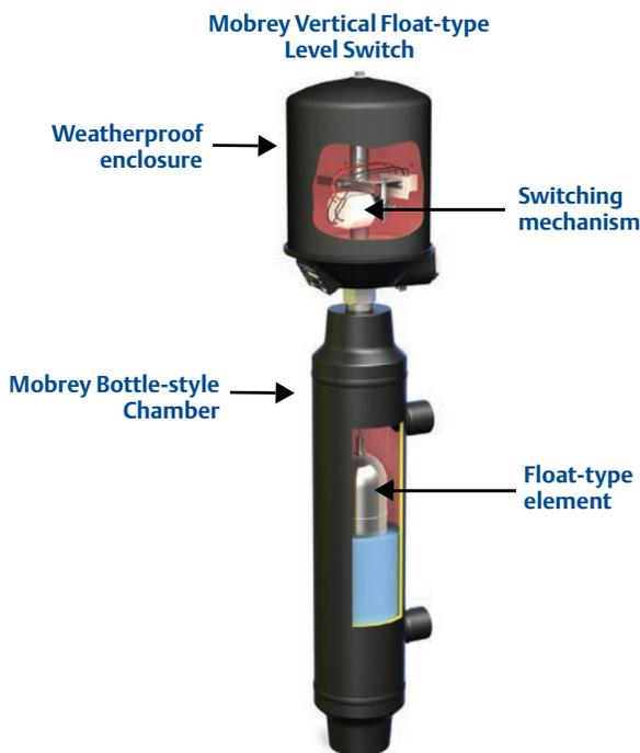
One or more switching mechanisms (see page 12) are mounted inside a weatherproof or flameproof enclosure. Switching is achieved with the unique Mobrey three-magnet system, giving reliable snap-action 'latch-on' switching.
