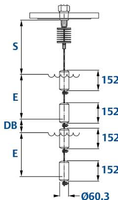
**Type 13D (two 4- or 8-contact switch mechanisms and wide switching differential)**
