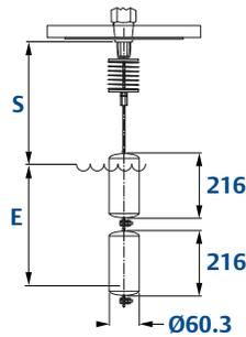
**Type 12D (one 4- or 8-contact switch mechanism and wide switching differential)**
