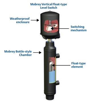
One or more switching mechanisms (see page 12) are mounted inside a weatherproof or flameproof enclosure. Switching is achieved with the unique Mobrey three-magnet system, giving reliable snap-action 'latch-on' switching.
