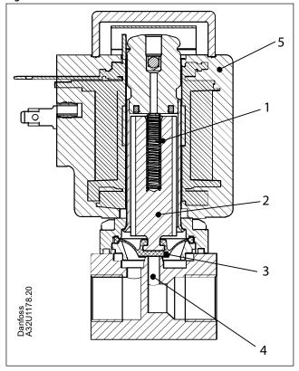
1. Closing spring 2. Armature 3. Isolating diaphragm 4. Orifice 5. Coil
