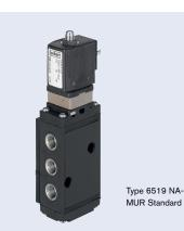
The valve bodies of Type 6519 NAMUR are identical with the Ex m variants. The difference is in the coils, which are laid out and approved in different ways. By changing the coil on the valve body, it is possible to easily convert from Non-Ex operation to Ex operation (or vice versa). The coils are designed to be push-over and can be locked in  $4 \times 90^{\circ}$  displaced positions and be positioned any where in-between.
