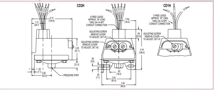
**Product Configurator** CD1H **3SS** Example -A \* Highlighted options represent those most frequently used. Select these common options for improved availability. (5/21) Hermetically sealed limit switch option - Class I, Division II Н (requires AA, CC, GH, HH limit switch, not available in
