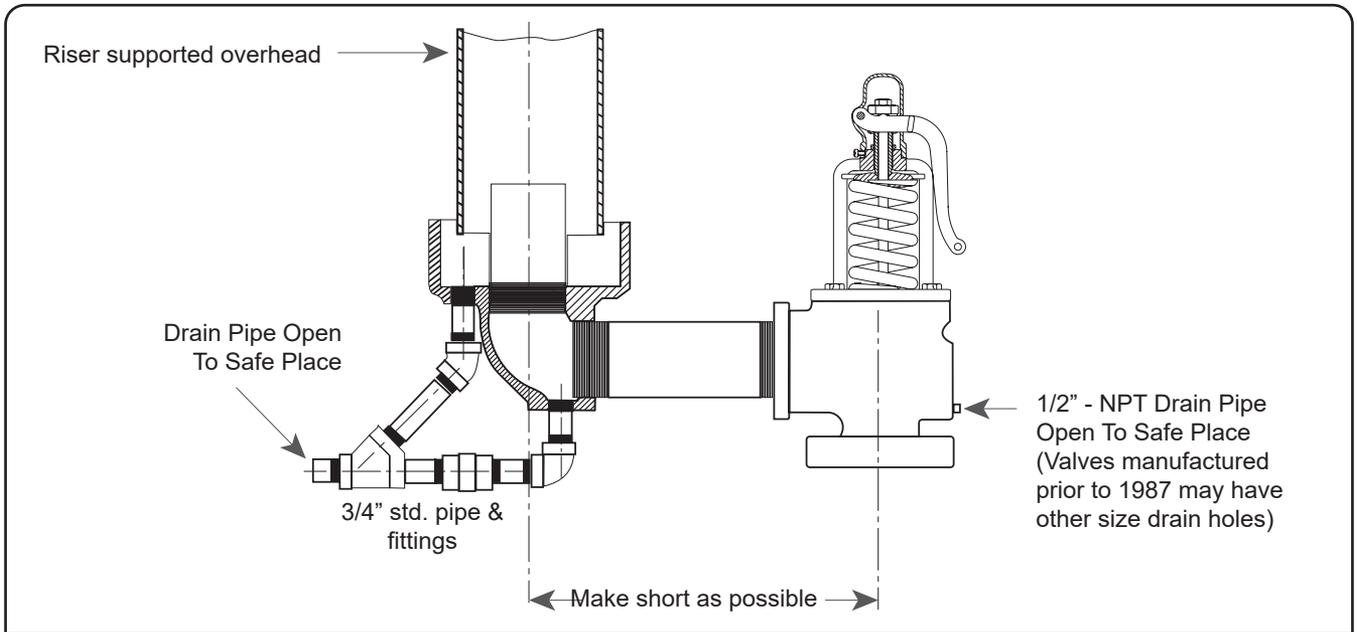
**Figure 3: Recommended Installation for Discharge and Vent Piping**
