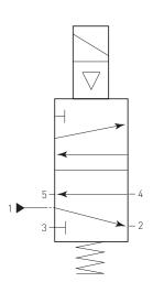
FIGURE 2 - SPRING RVETURN VALVE 4-WAY
