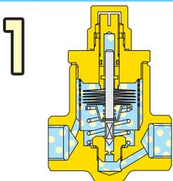
1 At startup, the bimetal element is contracted. The coil spring holds the valve open, quickly discharging the cold air and initial condensate.
