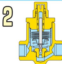
2 When the condensate temperature rises, the bimetal begins to expand. The valve begins to close, allowing less condensate to flow.
