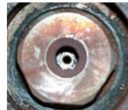
Not only is the obstruction removed from the orifice, but the surrounding valve seat surface is cleaned as well, a result of loosening the buildup followed by steam and condensate blowdown.
