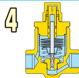
4 When the condensate temperature drops below the preset level, the element contracts. The coil spring opens the valve, allowing condensate to be discharged. Steps 3 and 4 alternate as condensate temperature changes.
