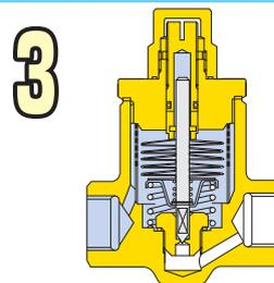
3 When the condensate reaches the preset temperature, the valve shuts tightly, stopping all condensate discharge.
