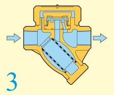
Eventually, the pressure chamber is cooled when condensate enters the space above, lowering the steam pressure in the pressure chamber and thus allowing the inlet pressure to push the disc up and discharge condensate. Entering flashing condensate/steam then closes the trap, as in step 2.
