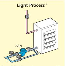
For applications where precise temperature control is necessary, free float type steam traps are recommended.
