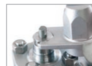
Tightening the gland retainer
