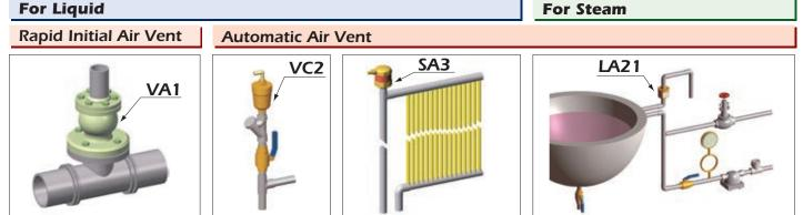
Note: • Inlet piping with no horizontal portion is recommended for water/air displacement. If there is a horizontal portion, make the pipe diameter of the horizontal portion larger than the vertical portion or make the horizontal portion as short as possible.
