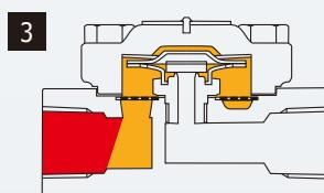
Just before the condensate reaches saturation temperature, the valve plate will close the seat completely. Steam can not enter the trap, ensuring zero steam loss.
