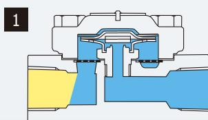
Upon start-up in the presence of cold condensate, the capsule element is contracted and the valve plate has moved away from the seat. The wide open valve discharges condensate and air rapidly.
