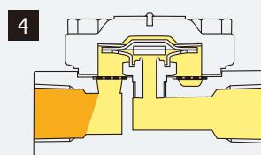
As the temperature inside the trap decreases, the capsule element moves away from the seat and the condensate will be discharged. During normal operation steps 3 and 4 will repeat continuously.
