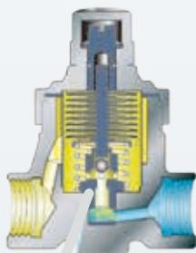
As the temperature of the condensate increases, the bimetal discs begin to curve gradually and force the valve shaft and the valve holder to move down.
