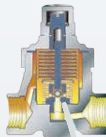
When condensate with higher temperature (near to set temperature) flows in, the bimetal discs are curved even more and, at the same time, the valve shaft moves down and the valve holder closes the holes in the guide partially.
