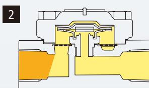
As the temperature inside the trap increases, the capsule element will start to expand, moving the valve plate toward the seat.
