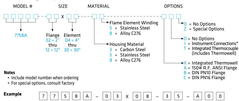
Indicates a 3" Model 7758A with Carbon Steel housing, 8" Stainless Steel Flame Element, ANSI Flanged Outlet and no other options.
