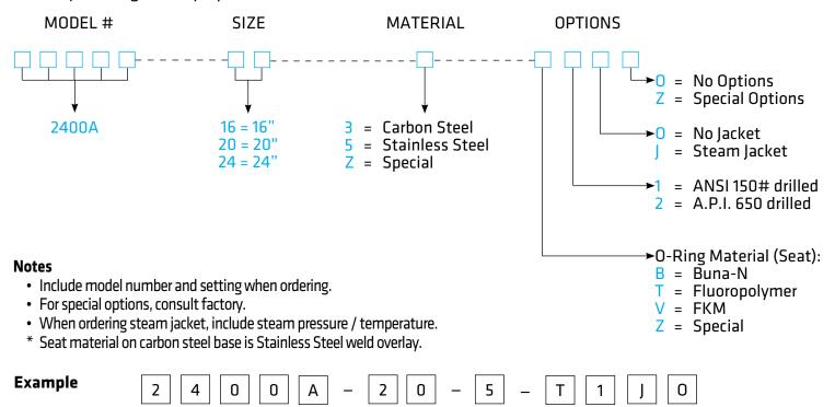
Indicates a 20" Model 2400A with Stainless Steel Body, Fluoropolymer Seat Diaphragm, ANSI 150# drilled, Steam Jacket and no other options.
