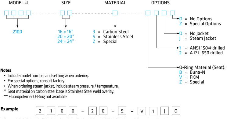
Indicates a 20" Model 2000A with Stainless Steel Body, FKM Seat O-Ring, ANSI 150# drilled, Steam Jacket and no other options.
