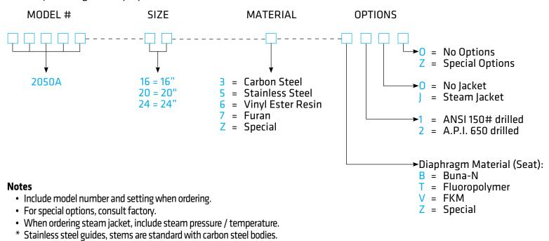
Indicates a 20" Model 2000A with Stainless Steel Body, Fluoropolymer Seat Diaphragm, ANSI 150# drilled, Steam Jacket and no other
