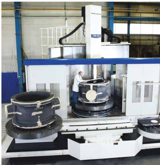
Two station CNC vertical borer with live spindle and tool changer
