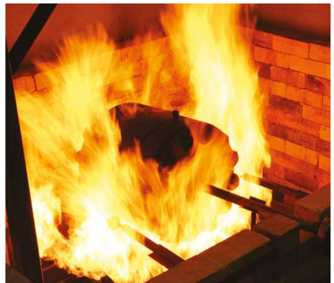
8" 1500# BSR Solid Lug Check Valve undergoing fire test
