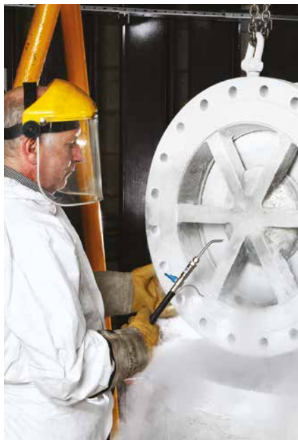
18" 300# Axial Check Valve Type NKF on Cryogenic Test
