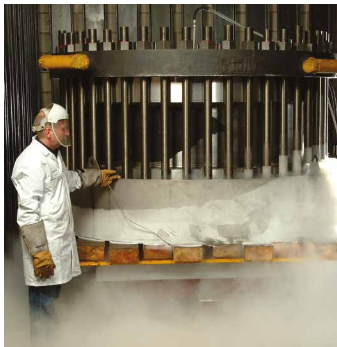
Cryogenic test facility for helium leak testing
