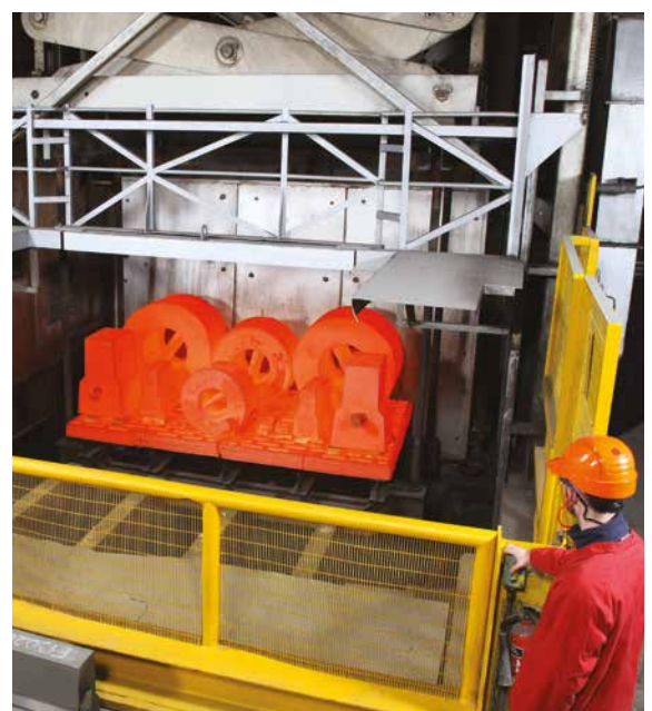
Super Duplex valve bodies with representative sized keel blocks undergoing heat treatment (From furnace to quenching in under 30 seconds)
