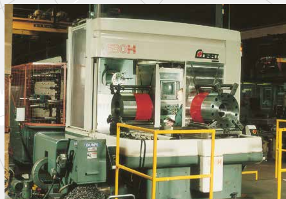
Twin pallet CNC machining centre with 60 tool changer
