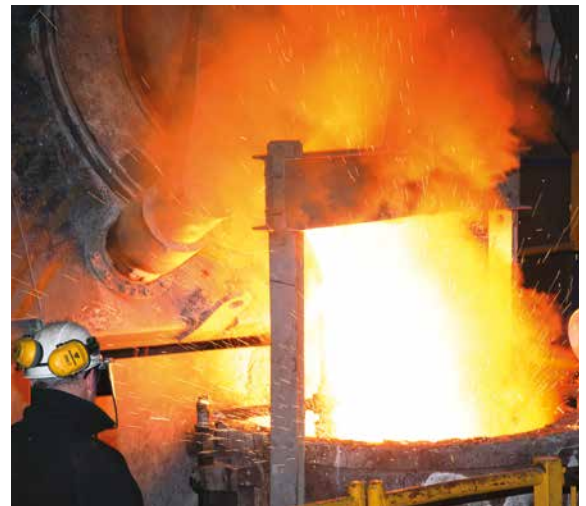
12 tonne induction holding furnace at Goodwin Steel Castings
