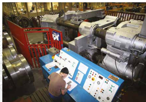
2500 tonne hydraulic test rig in Goodwin assembly bay
