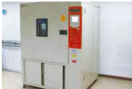
Constant Temperature and Humidity Test Chamber
