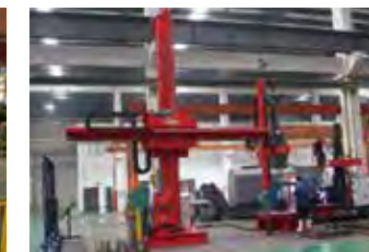
Hot-wire TIG Automatic Cladding System
