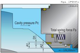
When force created by cavity pressure (Pc) is lower than the force created by line pressure (Pl), i.e.  $\triangle P^*D1 < Fs$ , then contact between ball and seat ring is assured to provide a tight seal.
