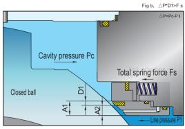
When cavity pressure is higher than seat spring force plus line pressure, i .e. P\*D1>Fs, the self relieving action allows the valve seat to move slightly away from the ball surface. Therefore, any overpressure inside the body cavity is discharged into the pipeline to restore thebalance between the body cavity and the pipeline (either upstream or downstream side).
