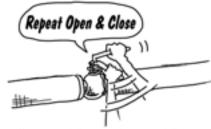
🙎 Be careful not to damage the seal part of ball surface and flange face during disassembling and assembling.
