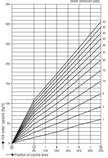
Fig. 2 For DN 15 to 32 Capacity range up to 310 kg/h
