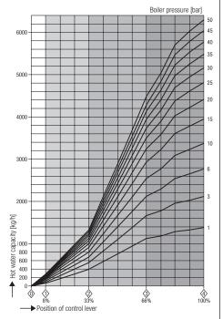
Fig. 5 For DN 40 and 50 Capacity ranges at a glance
